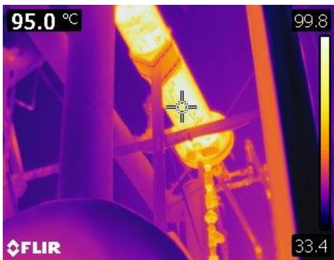
Figure 5 This thermographic image is of a pump located adjacent to Steam Pac 1. Also associated piping is not insulated at 74° C or 154° F
