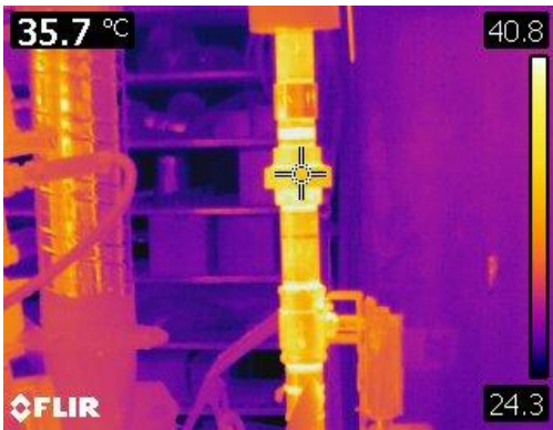
Figure 15 This thermographic image is of supply piping at top of boiler at 150° C or 302° F.
