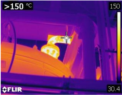
Figure 15 This thermographic image is of supply piping at top of boiler at 150° C or 302° F.
