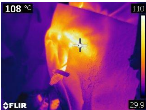
Figure 11 This thermo graphic image is of a motorized circulation pump at 150° C or 302° F.
