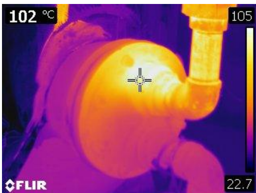
Figure 29 Thermographic image of the access hatch on vessel at 46° C or 114° F.
