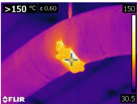
Figure 3 This is a thermographic image of an exposed valve bonnet at 115° C, or 239° F.
