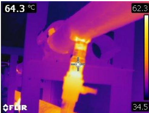
Figure 99 Thermographic image of improperly insulated piping where the outside surface temperature is 86.2° C or 187° F
