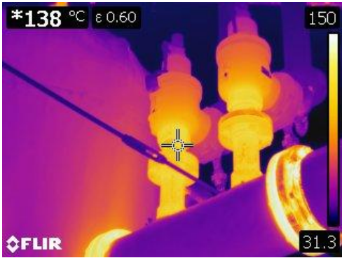
Figure 7 This is a thermographic image of a bare PSV at 138° C or 191° F.
