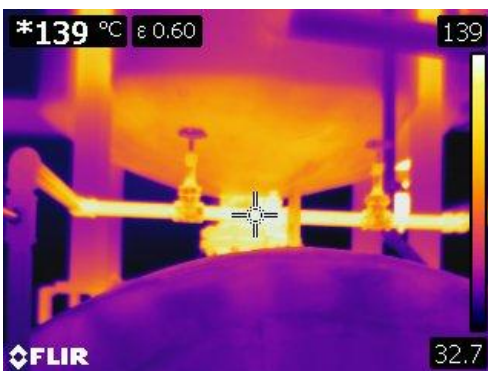
Figure 21 Thermographic image of a pipe support at a temperature greater than 150° C or >302° F.
