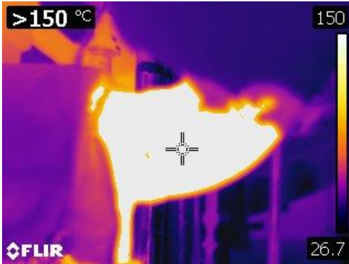
Figure 75 Thermographic image of an uninsulated elbow greater than 150° C or 302° F.
