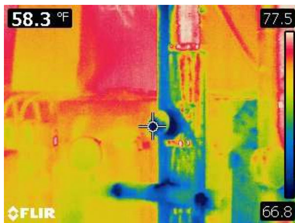
Infrared Image of Inadequate Chilled Water allowing moisture condensation
