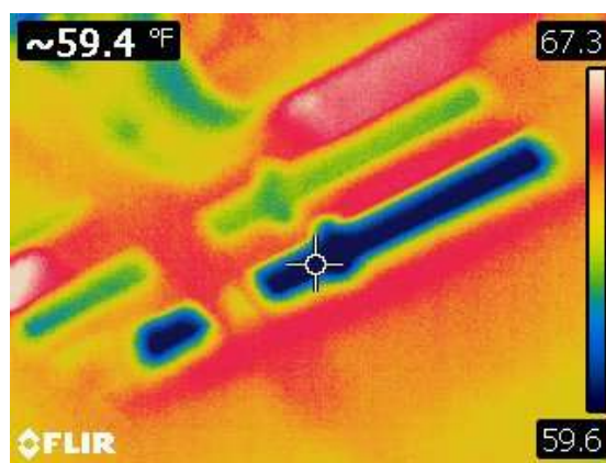
Infrared Image of Missing Thermal Insulation, allowing significant energy loss
