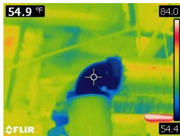
Infrared Image of Missing Thermal Insulation, significant energy loss – condensation issue & Corrosion Under Insulation (CUI)
