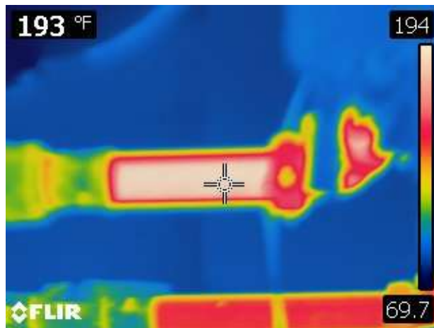
Infrared Image of Compromised Insulation due to Improper Support & Missing Insulation
