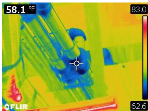
Infrared Image of Improper Insulation Installation, energy loss – condensation issue & Corrosion Under Insulation (CUI)
