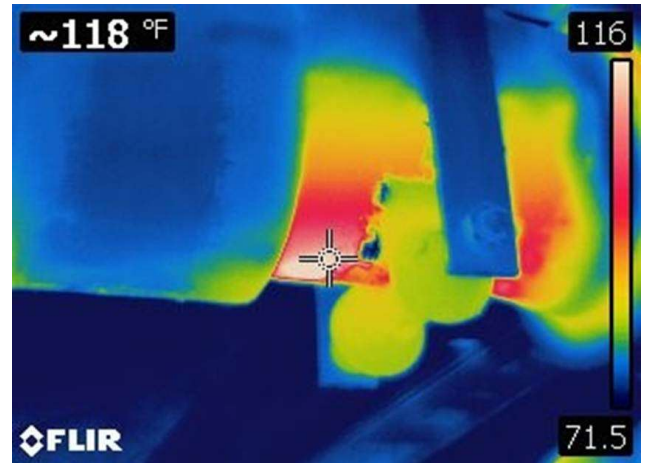
Infrared Image of Improper Support with Compromised Insulation
