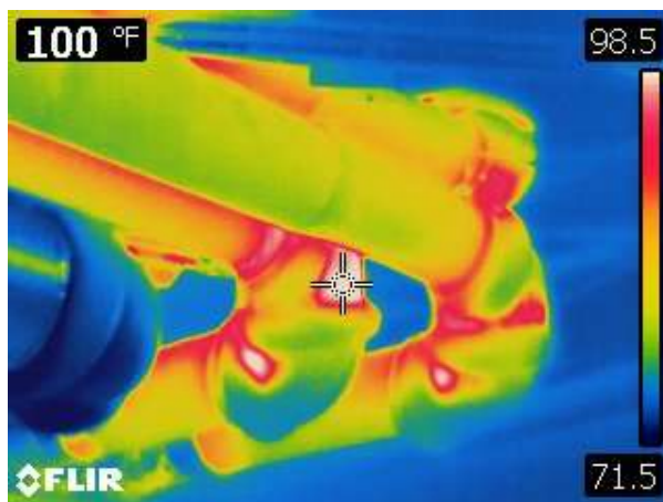
Infrared Image of Improper Thermal Insulation Installation, allowing significant energy loss, due to installation issues
