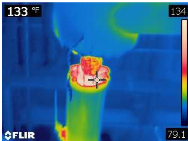
Infrared Image of Missing Domestic Hot Water Insulation Contributing to fluid temperature drop
